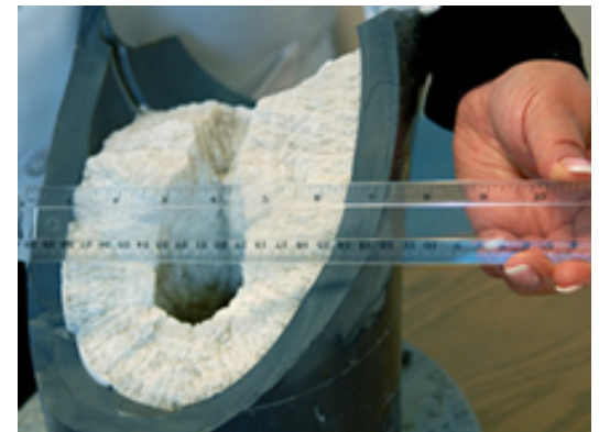
"Struvite Removed from Digesters to Restore Biosolids Treatment Capacity" http://www.dsrds.com/invest/reducecostincreaseefficiency.html (1 November 2011)
